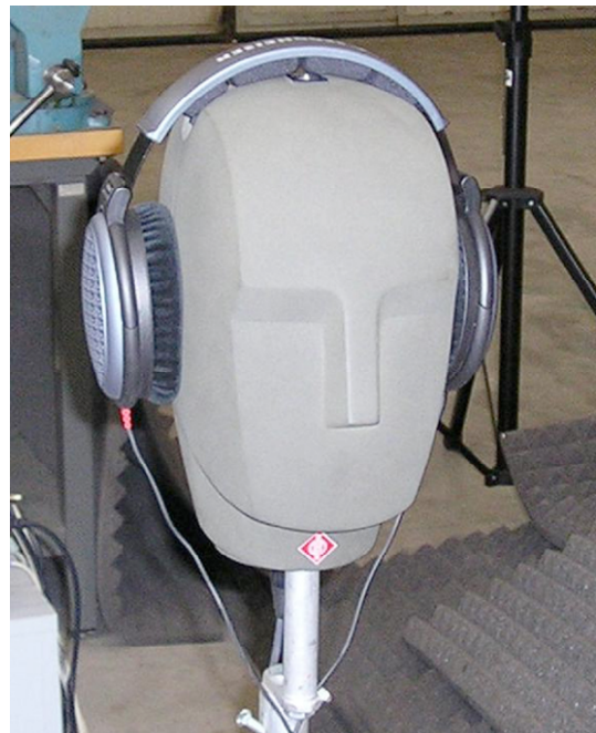
Fig. 14 – dummy head and headphones
